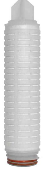
MICROPVDF pleated cartridge filters are made of polyvinylidene fluoride (PVDF) and are characterized by low protein binding, low extractable levels, wide chemical compatibility and chemical inertness. The pleat technology maximizes the useful surface area of the filter while maintaining proper flow paths between media pleats. Adaptors are thermally welded with media without using any adhesives on it, ensuring seamless fusion.
